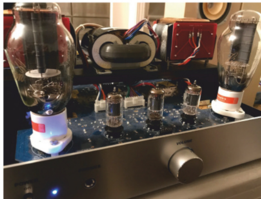
Left: An unfinished TU-8600R; note Lundahl output transformers straddling the mains transformer. Right: Farther along, with tubes in place.
